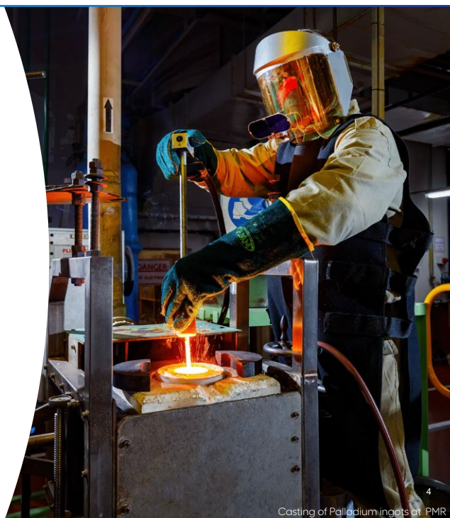
Casting of Palladium ingots at PMR
