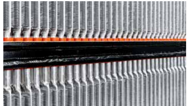
Close up of a fuel-cell electric vehicle (FCEV) haul truck's power plant radiator.
