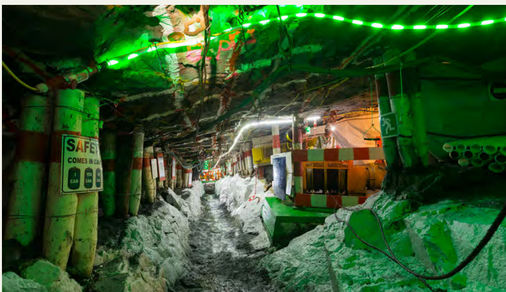
The winch signalling system has light sensors that detect LED lights on caplamps and automatically shuts down winches when a caplamp shines on it.
