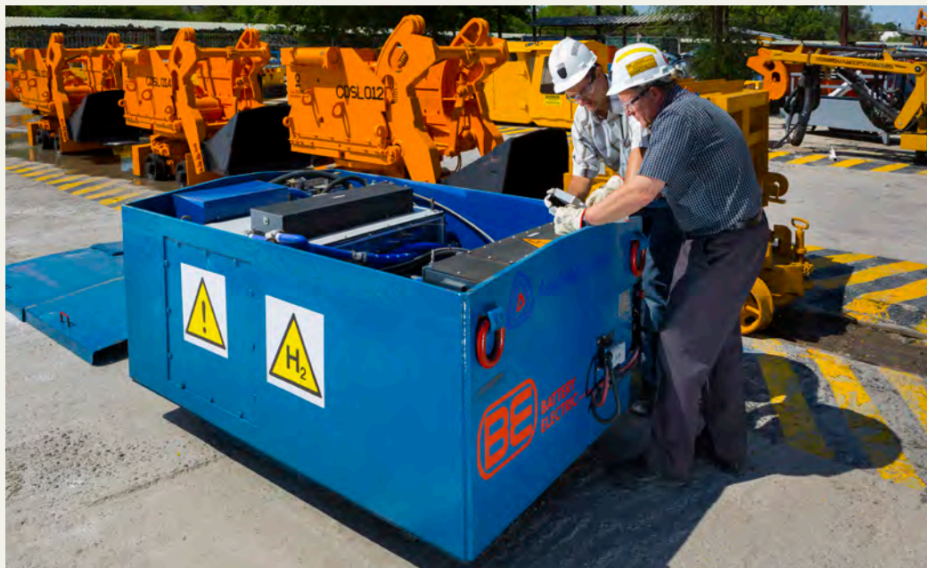
Hydrogen fuel cells for underground loco, being tested for fuel-cell stack voltage before being piloted at Tumela Mine
