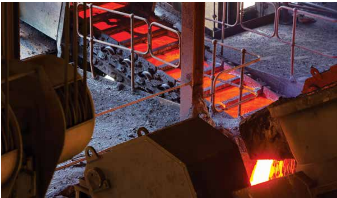
Image Furnace matte being cooled on the caster system at Polokwane Smelter.
