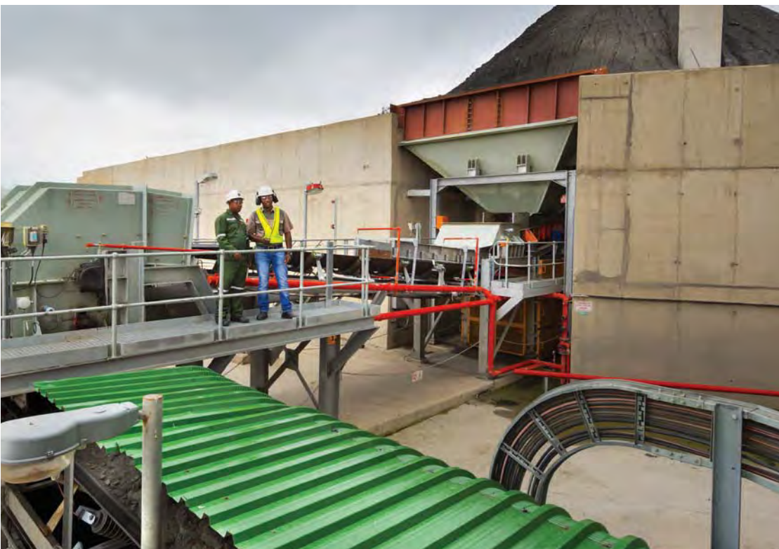
Kenny Fenyane (Process operator) and Muhle Boroko (Plant manager) inspecting the belt transfer on the stockpile conveyors at Mototolo Concentrator.
