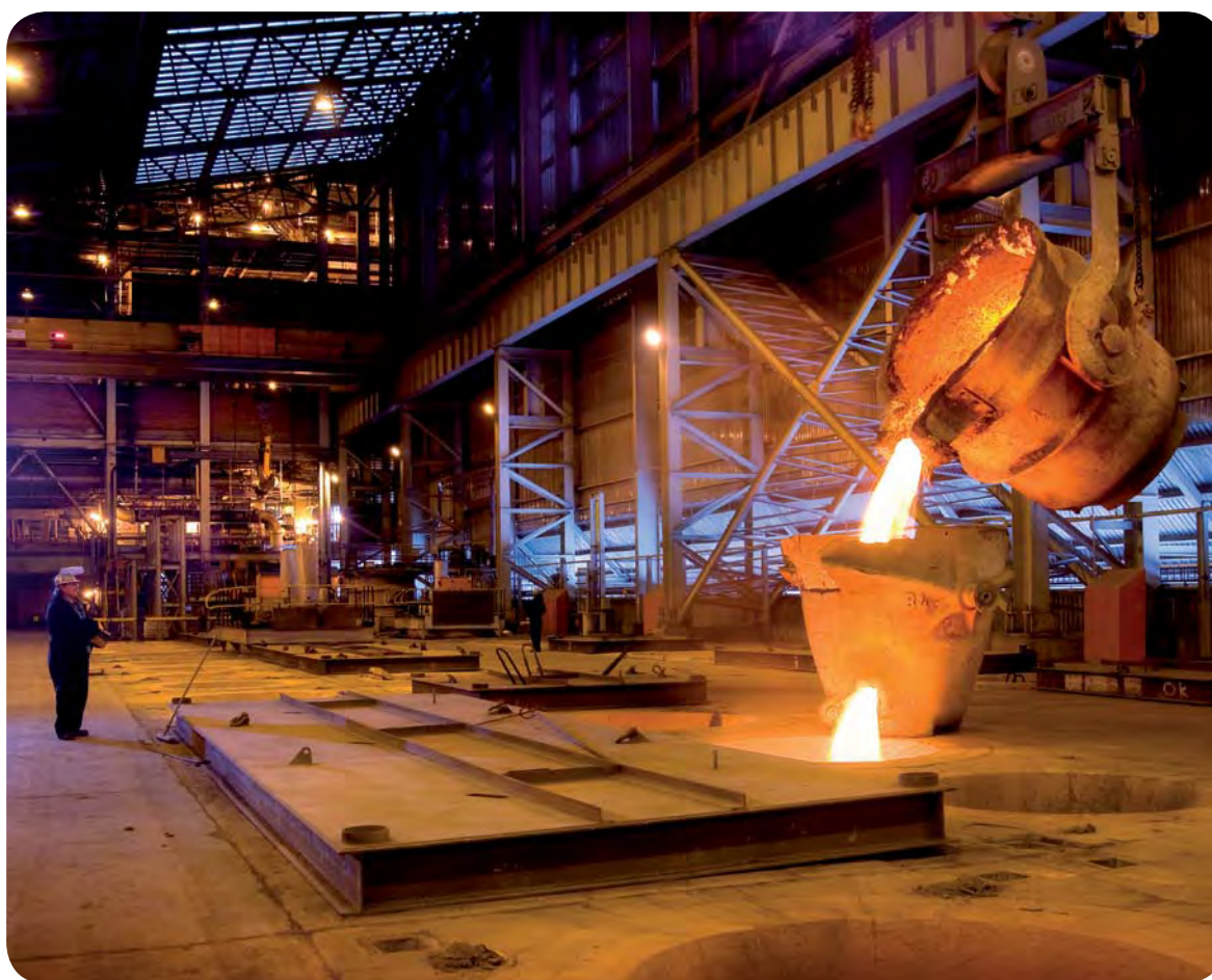
ACP matte being poured into a slow-cool mould
