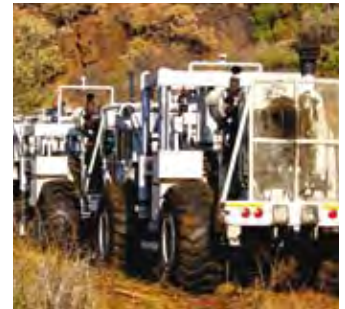
A convoy of seismic vibrator trucks at the Modikwa joint venture. The technique is used to image subsurface structure, assisting in geological modelling and mine planning.
