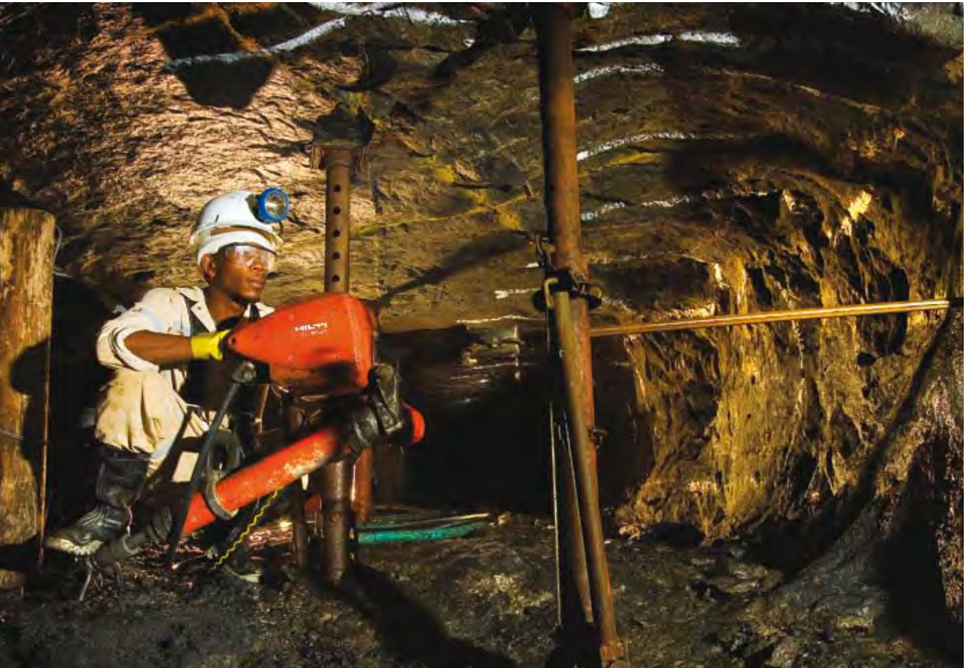
Tsheph Tladi operates an electric drill in a stope at Brakspruit shaft
