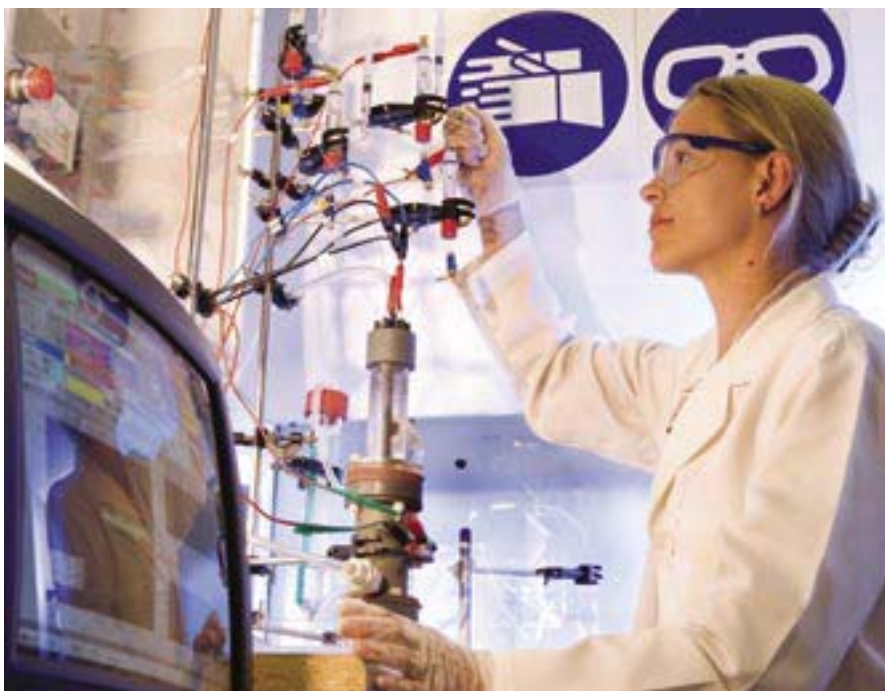
Bronwynne Ferreira, a senior metallurgist at ARC working on the Electrochemical Reactor, a new technology used in the recovery of PGMs from effluent.
