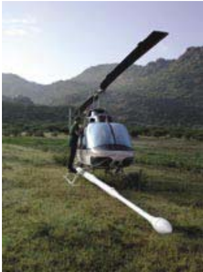
MIDAS helicopter borne aeromagnetic survey system
