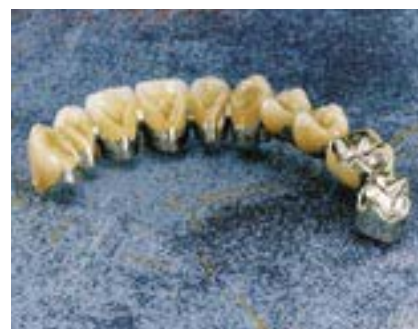
Palladium-based alloys, compatible with human tissue, are used in dentistry for dental crowns and bridges.
