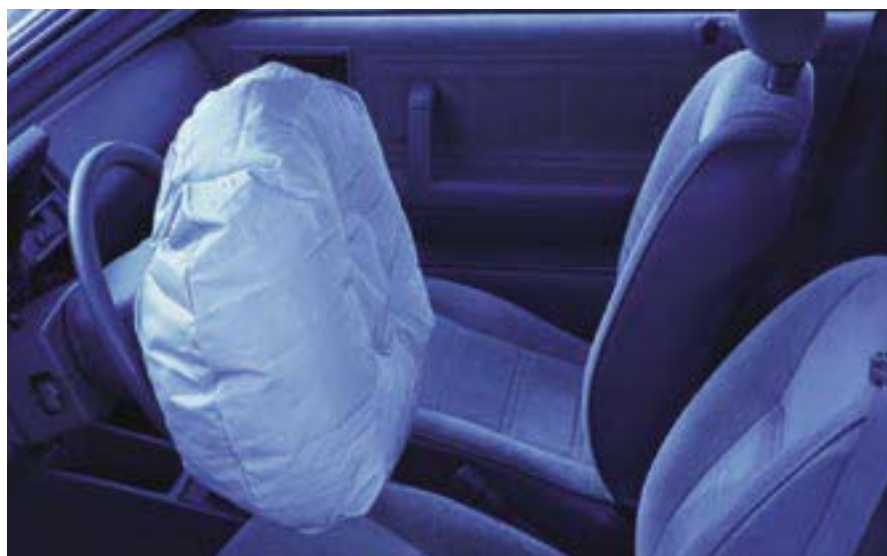
'Airbag initiators may be used only once and after long periods of inaction. So the electronic components that make them work must be durable and reliable which is why platinum, with its corrosion resistance, durability and conductivity is used'.
