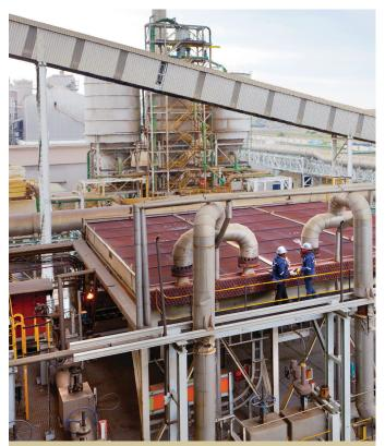
The existing high-pressure cooling system at Waterval Smelter from which hot water will be diverted for use in power generation. In the shot are Xolisile Mahlangu (Processor) and Mbanza Sichone (Metallurgical Technical Engineer)
