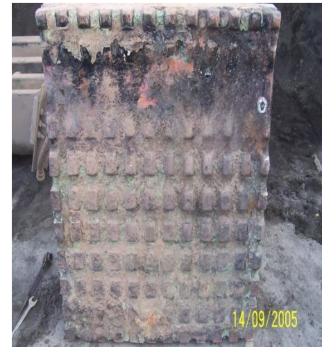
Copper coolers with graphite lining
