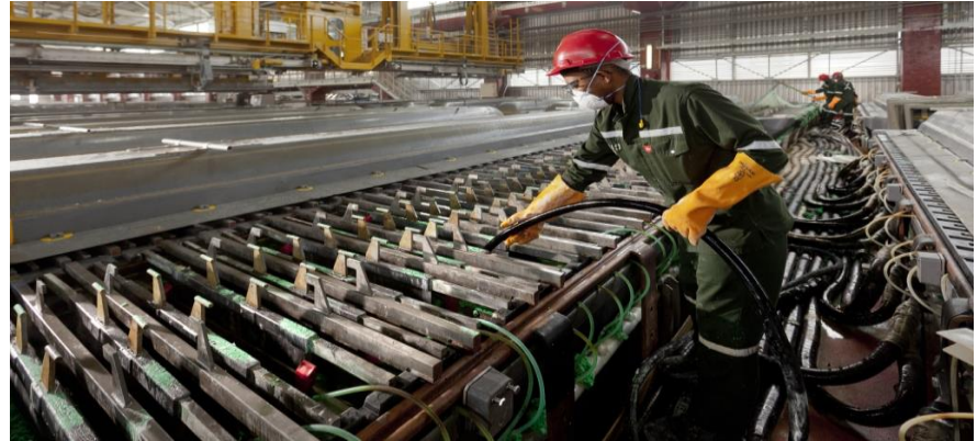
Process Operator conducting manual cathode bag top-up with nickel feed after cell harvesting
