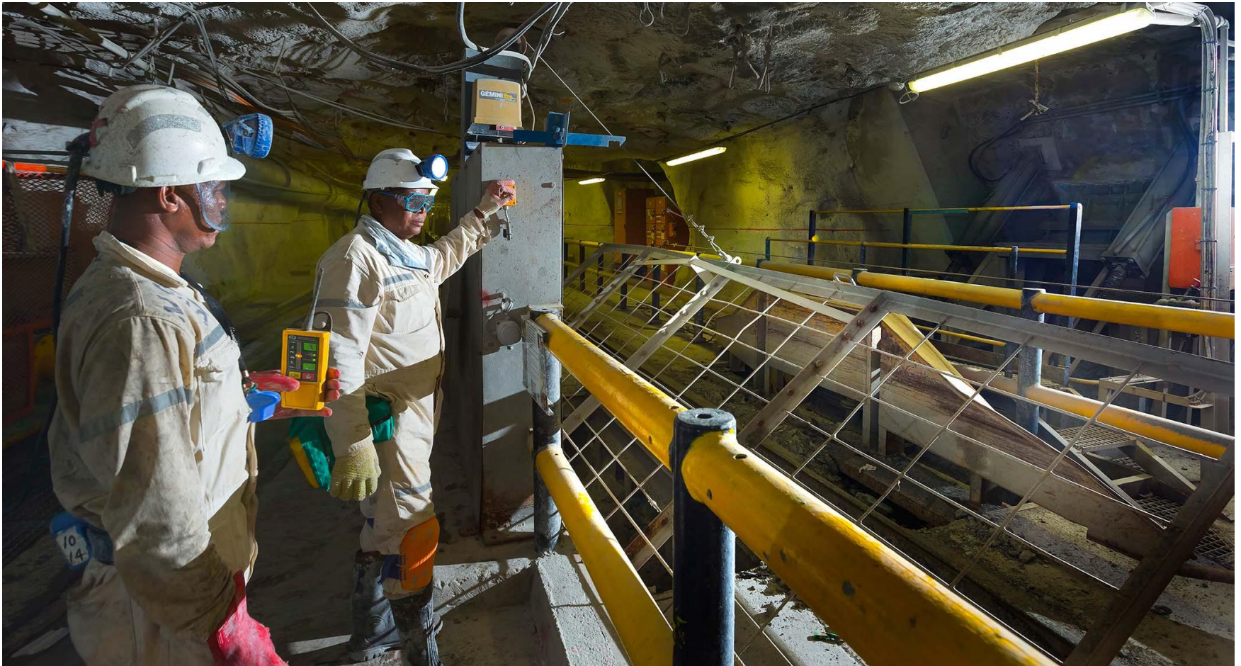
An operator closing the main shaft ore pass tip cover (a safety device to ensure persons cannot fall into the ore pass)
